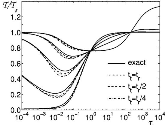
FIG. 1. Relative mean escape time  $\mathcal{T}/\mathcal{T}_s$  versus  $\tau$  for DN case with a triangle barrier  $U(x)=10(1-|x|)$  and  $V(x)=1-|x|$  confined to the interval  $(-1,1)$  for  $Q_0=1$ ,  $q=1$ ,  $x_{thr}=0$ ,  $t_r=0.09$ , and  $\alpha=0, 0.25, 0.50, 0.75$ , and  $1.0$  from the bottom to the top on the left-hand side, respectively. Solid lines show the exact results and the others the approximation (13) for few values of  $t_t$ .
