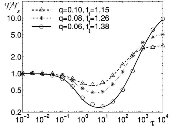
FIG. 2. Relative mean escape time  $\mathcal{T}/\mathcal{T}_s$  versus  $\tau$  for OUN case and the system with  $U(x)=x^4/4-x^2/2$ ,  $V(x)=U(x)+1/4$  for  $|x| \leq 1$ , and  $V(x)=0$  elsewhere, for  $q=0.08$ ,  $Q_0=0.8$ ,  $t_t=t_r/2=1.26$ , and three values of  $\alpha$ . The lines present our approximation and markers are from the numerical simulation of Eq. (1).
